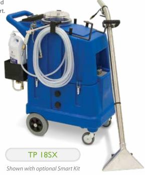
The TP 18SX is a premium extractor featuring a 130 psi pump with 1.2 gpm of water flow. The 18 gallon polyethylene tanks are designed to clean large areas and it comes complete with a 20' solution/vacuum hose and three-jet wand.
